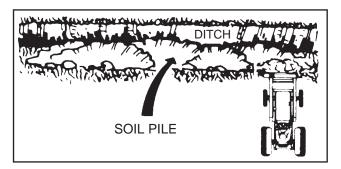
Operate at right angles to the ditch. Take as big a bite as the tractor can handle without lugging down.
